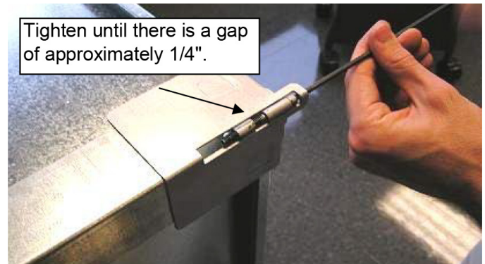
Figure 46: Tighten Cap Screw to 1/4" of the Coupling
